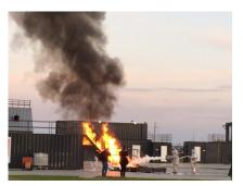
2. Cascade of burning stairs: an exercise to simulate skills of extinguishing the cascade of burning stairs using foam.
